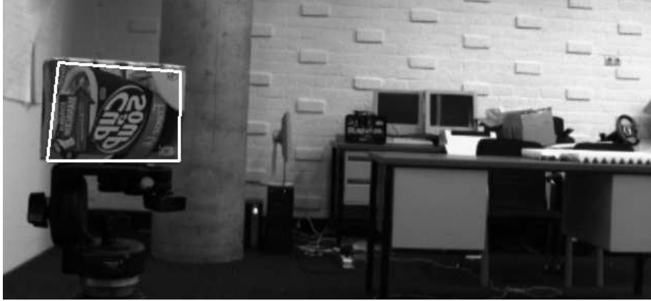
Figure 8.5: Surf feature detector executed in an office environment. The obstacle is detected and outlined with a white rectangle.
