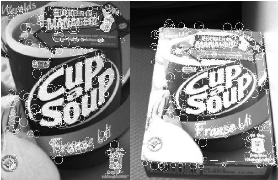
Figure 4.6: Example of SURF detector and descriptor. A relatively large number of false positive keypoints are detected which are discarded via the keypoint matching process. Despite the difference in image intensity, the reference image is found in the current image, as is indicated by the white rectangle.
